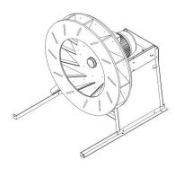
2. Place plastic back plate and impeller onto shaft with TaperLock bush and tighten
