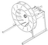
2. Place plastic back plate and impeller onto shaft with TaperLock bushing and tighten.
