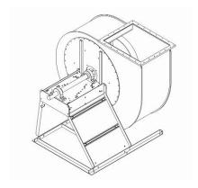
3. Join casing with round steel plate together with bolts
