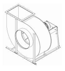
4. Screw bracket to base frame. Mount casing reinforcements to bracket
