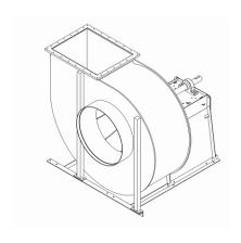
4. Screw bracket to base frame. Screw casing reinforcements to bracket.
