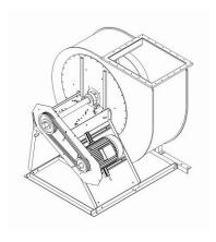
5. Mount sliding rails, steel part of V-belt protection and V-belt drive.
