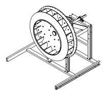
2. Fit rear panel to support. Slide impeller on drive shaft.
