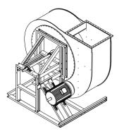
3. Screw housing to fan rear panel.
