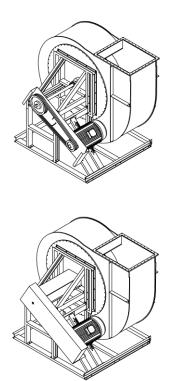
5. Fit V-belt protection panel and V-belt drive.
