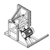
Screw individual parts of fan support together. Fit bearing units and shaft on support. Fix motor to support.
