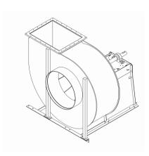
4. Screw bracket to base frame. Screw casing reinforcements to bracket.
