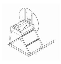
1. Attach support steel sheets including round steel plate, pedestal bearing and shaft to base frame.
