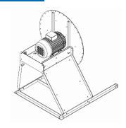
1. Attach support steel sheets including round steel plate and motor to base frame.
