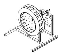
2. Fit rear panel to support. Slide impeller on drive shaft.
