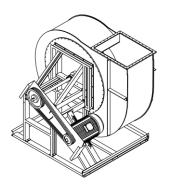
5. Fit V-belt protection panel and V-belt drive.
