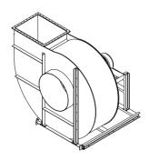
4. Screw bracket to base frame. Fit housing brace at front and rear. Position impeller, tighten and fit hub cap.
