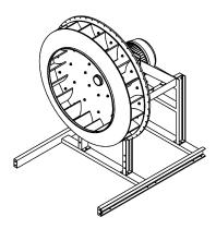
2. Fit rear panel to support. Slide impeller onto shaft.
