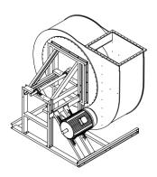
3. Screw housing to fan rear panel.
