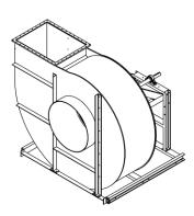
4. Screw bracket to base frame. Fit housing brace at front and rear. Position impeller, tighten and fit hub cap.
