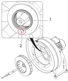
Fig. 43: Replacing the V-ring seal
