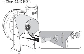
Fig. 36: Mounting the motor cover (DD)
