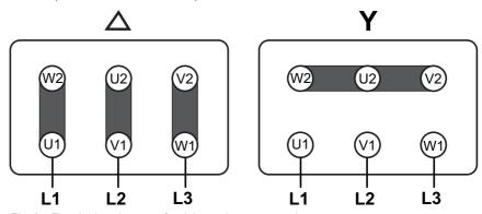
Fig. 35: Terminal assignment for delta and star connection
