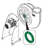
Fig. 17: Hub seal felt ring
