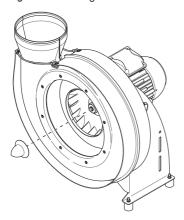
Fig. 38: Removing hub cap
