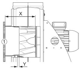
Fig. 42: Measuring impeller position (sectional view)
