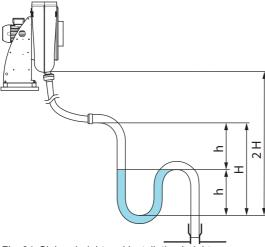
Fig. 31: Siphon height and installation height
