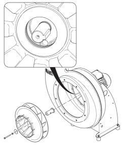
Fig. 44: Replacing the felt ring of the hub seal
