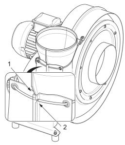
Fig. 24: Proper mounting of the splinter protection
