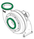
Fig. 8: Flange connections
