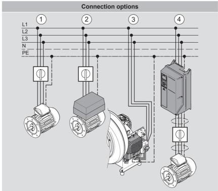
Depending on the execution, an electric motor can either be connected directly (1) to the electrical mains or can/shall be operated with a FC.
