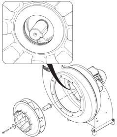
Fig. 41: Inserting hub seal
