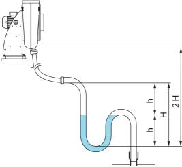
Fig. 29: Siphon height and installation height
