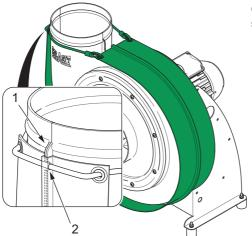
Fig. 22: Proper mounting of the splinter protection
