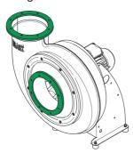
Fig. 8: Flange connections
