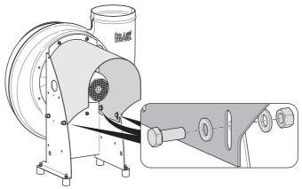
Fig. 34: Mounting motor cover
