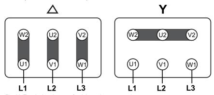
Fig. 33: Terminal assignment for delta and star connection
