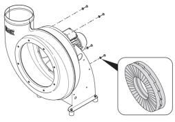
Fig. 38: Removing casing
