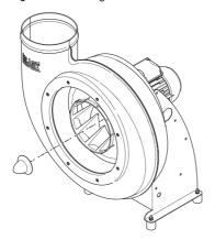
Fig. 36: Removing hub cap
