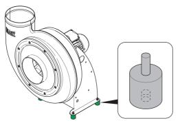
Fig. 4: Vibration absorbers for floor and wall mounting
