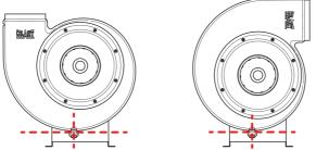
Fig. 28: Proper position of the casing drain
