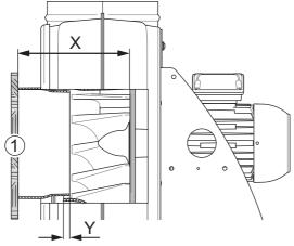
Fig. 40: Measuring impeller position (sectional view)
