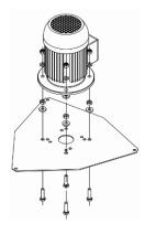
1. Attach motor to the motor plate
