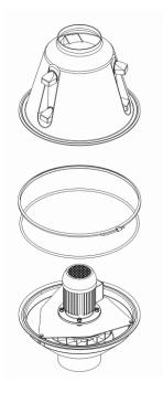
4. Mount round seal an upper part of housing on the lower part, fasten both housing halves together using the retaining ring
