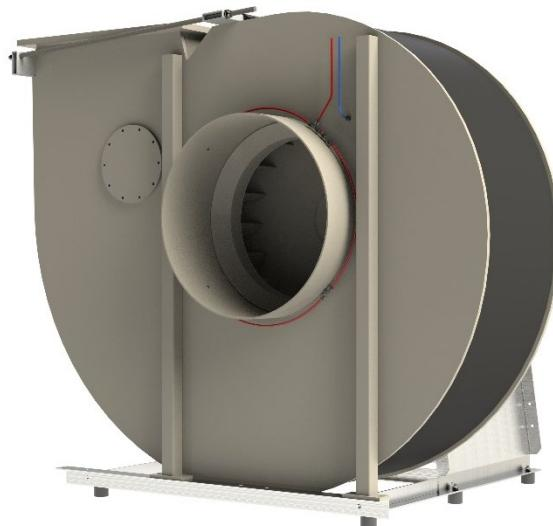
The differential pressure  $\Delta p$  is measured upstream and downstream of the measuring point (red = overpressure, blue = negative pressure). The differential pressure correlates with the volume flow. To calculate the volume flow, the calibration factor "k" for the respective fan type is used together with the density of the medium in the formula below:
